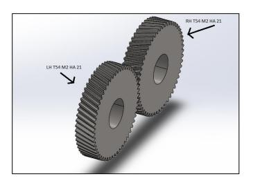
Fig-2: Helical gear assembly in solid works
