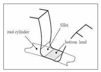
Fig-3: Root fillet radius in a gear
