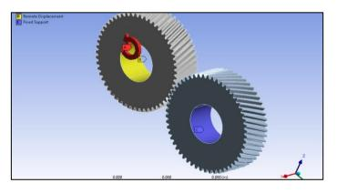
Fig-5: Boundary conditions of gear model.
