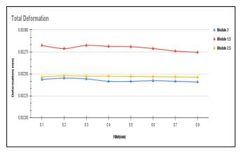
Fig-9: Total Deformation vs root fillet radius
