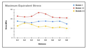
Fig-8: Maximum Equivalent Stress vs root fillet radius
