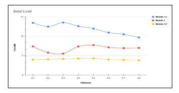
Fig-11: Axial load vs root fillet radius
