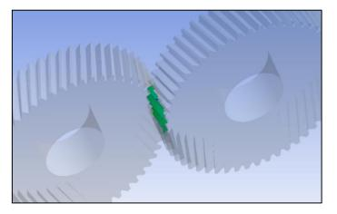
Fig-7: Contact Stress in helical gears
