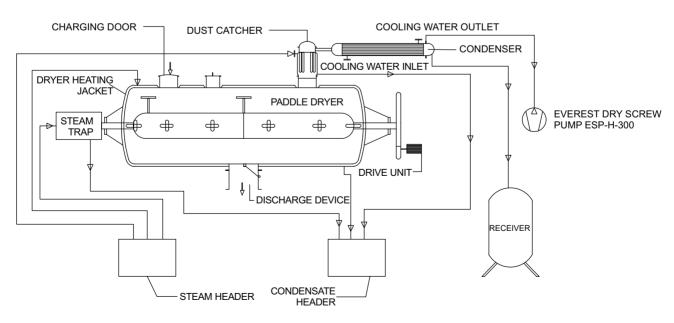
Rotary Baffle Dryer Used For Solvent Recovery
