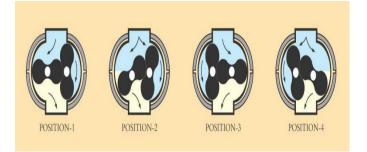
Fig -5: Rotary Lobe Vacuum pump
