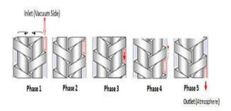
Fig -6: Phases of dry pump operation
