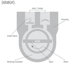
In the case of gas ballast operation, a hole to the outside is opened, which empties into the sealed suction chamber on the front side. As a result, the pressure needed to open the outlet valve is attained at relatively low compression during the compression pumping phase. This allows a displaced gas/vapor mixture to be expelled before the vapor starts to condense. The final pressure reached during operation with gas ballast is higher than in operation without gas ballast.
