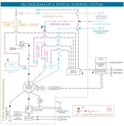
STANDARD SUPPLY | Screw Pump, Motor, VFD, Seal-Purge, Cooling Water Module (Standard), Non-Return Valve, Main Isolation Valve
