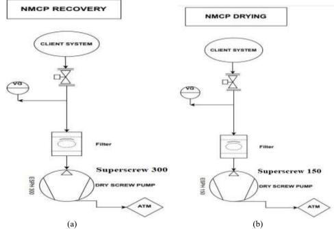
Fig 2: (a) Distillation & (b) Drying operation of N Methyl 4 ChloroPiperidine using Dry Screw Vacuum Pump
